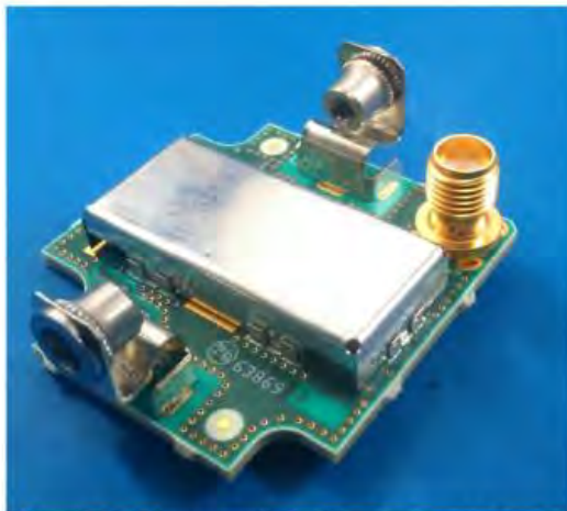
Figure 7-48: LNA prototype board showing 2-off feedtags to connect to the antenna elements and SMA connector to the FEM
